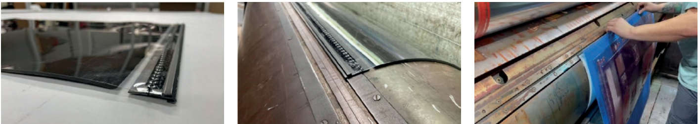
Figure 4: Foam blanket image; foam blank mounted on the cylinder; and with the plate.
